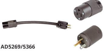
Edison Female/ Straight Blade/ Hubbell 5269EBK/ NEMA 5-15R, 15 Amp to Edison Male / Straight Blade/ Hubbell 5366EBK/ NEMA 5-20P, 20 Amp. Cable is 12/3 SOOW, 12" length. Custom lengths, colors and cable types are available.
