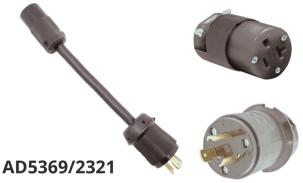
Edison Female/ Straight Blade/ Hubbell 5369EBK/ NEMA 5-20R, 20 Amp to Twist Lock Male/ Hubbell 2321/ NEMA L6-20P, 20 Amp, 250 Volt. Cable is 12/3 SOOW, 12" length. Custom lengths, colors and cable types are available. Call or email for pricing.
