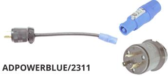
PowerCON Blue type, Locking, Power-in to Twist Lock Male/ Hubbell 2311/ NEMA L5-20P, 20 Amp, 125 Volt. Cable is 12/3 SJOOW, 12" length.
