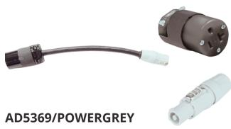
Edison Female/ Straight Blade/ Hubbell 5369EBK/ NEMA 5-20R, 15 Amp to PowerCON Grey type, Lockable, Power-out. Cable is 12/3 SJOOW, 12" length. Custom lengths, colors and cable types are available. Call or email for pricing.
