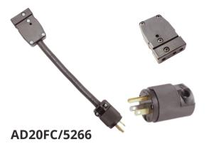
Stage Pin, Female, 20 Amp to Edison Male/ Straight Blade/ Hubbell 5266EBK/ NEMA 5-15P, 15 Amp. Cable is 12/3 SOOW, 12" length.
