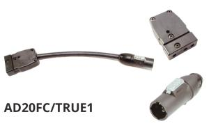
Stage Pin, Female, 20 Amp to PowerCON TRUE1 type, Locking Male. Cable is 12/3 SJOOW, 12" length.
