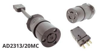
Twist Lock Female/ Hubbell 2313BK/ NEMA L5-20R, 20 Amp, 125 Volt to Stage Pin, Male, 20 Amp. Cable is 12/3 SOOW, 12" length. Custom lengths, colors and cable types are available. Call or email for pricing.
