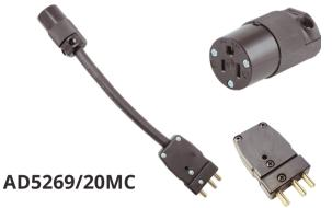
Edison Female/ Straight Blade/ Hubbell 5269EBK/ NEMA 5-15R, 15 Amp to Male Stage Pin, 20 Amp. Cable is 12/3 SOOW, 12" length.
