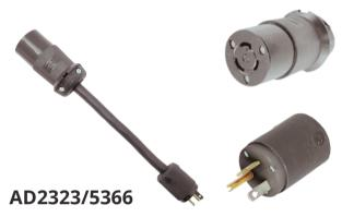
Twist Lock Female/ Hubbell 2323BK/ NEMA L6-20R, 20 Amp, 250 Volt to Edison Male/ Straight Blade/ Hubbell 5366EBK/ NEMA 5-20P, 20 Amp.
