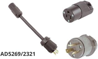
Edison Female/ Straight Blade/ Hubbell 5269EBK/ NEMA 5-15R, 15 Amp to Twist Lock Male/ HBL2321/ NEMA L6-20P, 20 Amp, 250 Volt. Cable is 12/3 SOOW, 12" length. Custom lengths, colors and cable types are available. Call or email for pricing.
