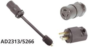
Twist Lock Female/ Hubbell 2313BK/ NEMA L5-20R, 20 Amp, 125 Volt to Edison Male/ Straight Blade/ Hubbell 5266EBK/ NEMA 5-15P, 15 Amp. Cable is 12/3 SOOW, 12" length. Custom lengths, colors and cable types are available. Call or email for pricing.
