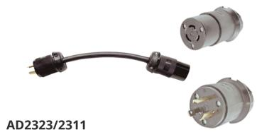
Twist Lock Female/ Hubbell 2323BK/ NEMA L6-20R, 20 Amp, 250 Volt to Twist Lock Male/ Hubbell 2311/ NEMA L5-20P, 20 Amp, 125 Volt.
