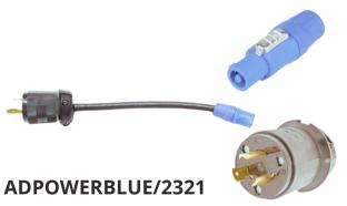
PowerCON Blue type, Locking, Power-in to Twist Lock Male/ Hubbell 2321/ NEMA L6-20P, 20 Amp, 250 Volt. Cable is 12/3 SJOOW, 12" length.
