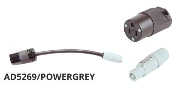
Edison Female/ Straight Blade/ Hubbell 5269EBK/ NEMA 5-15R, 15 Amp to PowerCON Grey type, Lockable, Power-out. Cable is 12/3 SJOOW, 12" length. Custom lengths, colors and cable types are available. Call or email for pricing.
