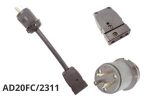
Stage Pin, Female, 20 Amp to Twist Lock Male/ Hubbell 2311/ NEMA L5-20P, 20 Amp, 125 Volt. Cable is 12/3 SOOW, 12" length. Custom lengths, colors and cable types are available.
