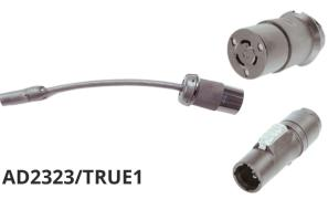
Twist Lock Female/ Hubbell 2323BK/ NEMA L6-20R, 20 Amp, 250 Volt to PowerCON TRUE1 type, Locking Male. Cable is 12/3 SJOOW, 12" length.
