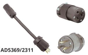
Edison Female/ Straight Blade/ Hubbell 5369EBK/ NEMA 5-20R, 20 Amp to Twist Lock Male/ Hubbell 2311/ NEMA L5-20P, 20 Amp, 125 Volt. Cable is 12/3 SOOW, 12" length. Custom lengths, colors and cable types are available. Call or email for pricing.
