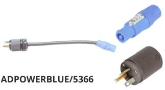
PowerCON Blue type, Locking, Power-in to Edison Male/ Straight Blade/ Hubbell 5366EBK/ NEMA 5-20P, 20 Amp.
