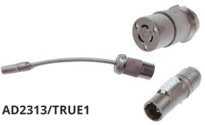
Twist Lock Female/ HBL 2313BK/ NEMA L5-20R, 20 Amp, 125 Volt to PowerCON TRUE1 type, Locking Male. Cable is 12/3 SJOOW, 12" length.
